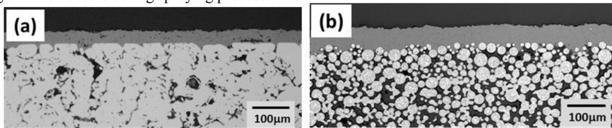
Fig. 1 Micrograph of LSCF coating deposited on porous Hastelloy X (a) and NiCoCrAlY (b) supports
