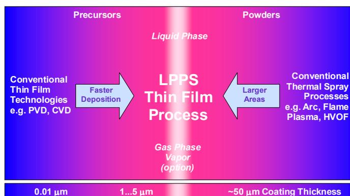
It is expected that, by using the PS-TF process, a dense, stable deposit with thickness lower than 20 micron can be obtained. This would allow increasing membrane performances while decreasing their manufacturing costs. Catalytic layers will be also applied to enhance the surface reactions becoming rate limiting for thin membranes.
