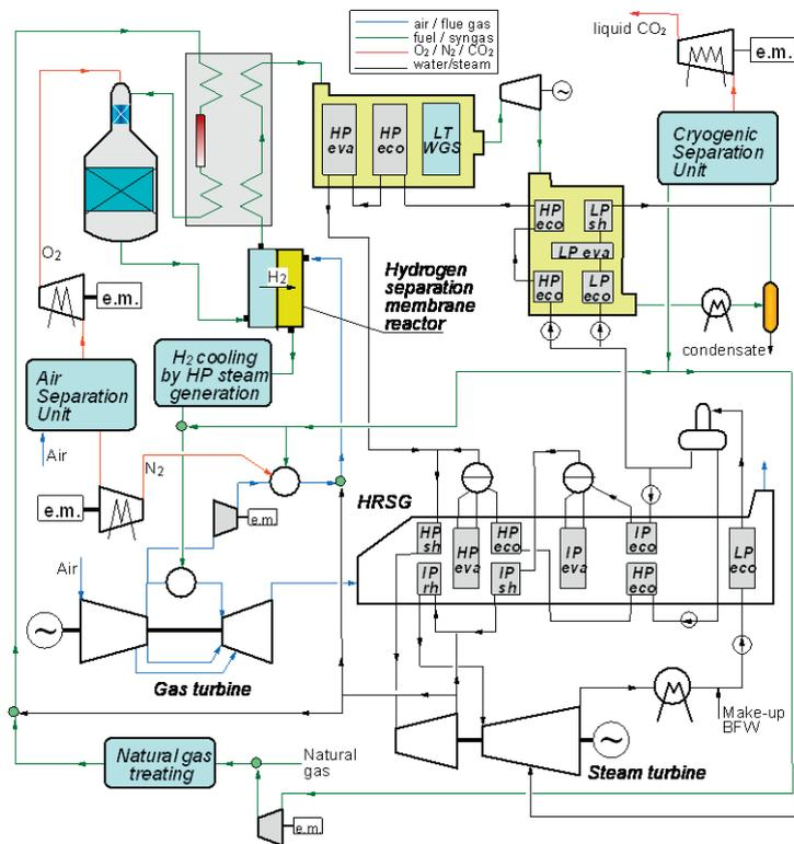
Fig.3 – Plant flow diagram of the ARHS configuration.
