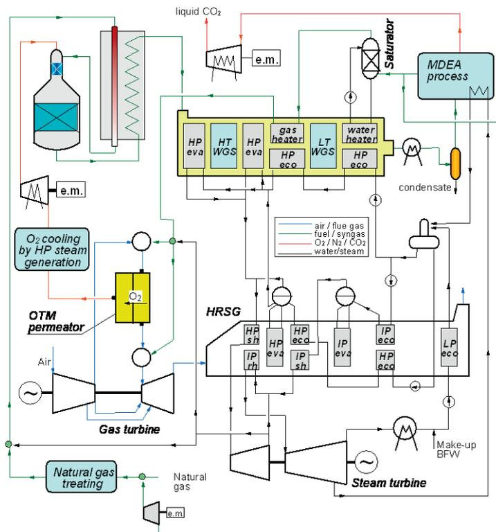
Fig. 1 – Plant flow diagram of the OMAR configuration.
